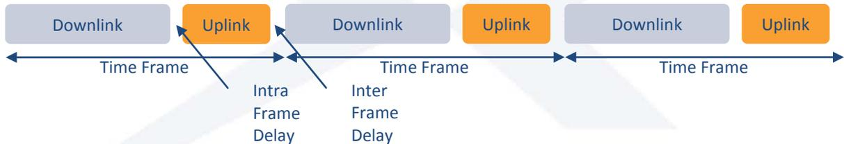
The benefit of TDMA is that if multiple base stations use the same values for Inter and Intra frame delays, as well as the same length time frame and uplink/downlink ratio then it is possible to synchronize these base stations so they are in transmit or receive mode simultaneously and thus greatly mitigate the issue of self interference for a dense deployment of BSUs. The graphic below shows how multiple BSUs with the same timing can operate “in sync.”
