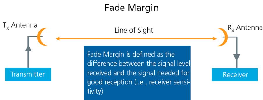
Fade Margin = Rx signal (dBm) - R<sub>x</sub> sensitivity (dBm)
