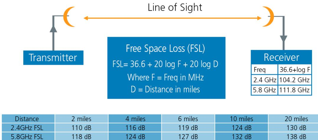
Rule of Thumb: Double / halve the distance - Add/Subtract 6 dB.
