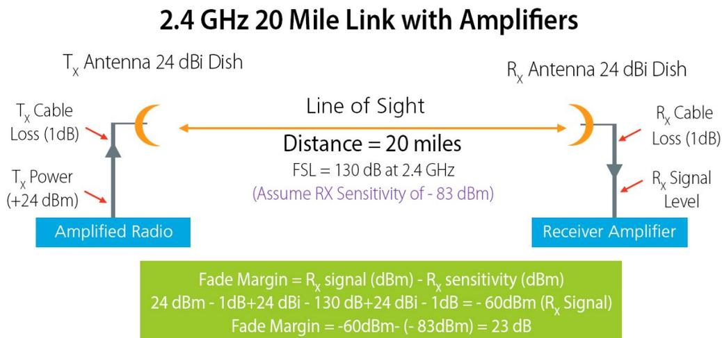
other properly (i.e., they are in each others' main lobe). To calculate Fade Margin in the example, start with the transmit power (+24 dBm), subtract the coax cable loss (1 dB) and add the transmit antenna gain (24 dBi). This gives you the effective isotropic radiated power:
