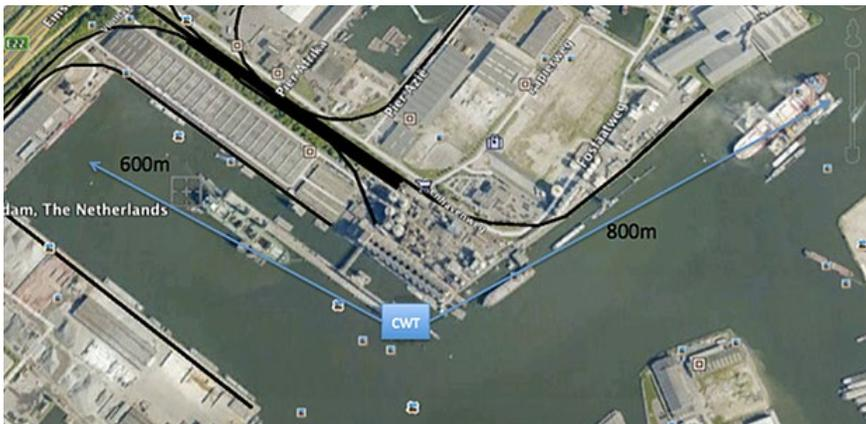
To cover the distance from the central weighing tower to both docks, two Tsunami® 8200 Base station units with 16.5dBi, 60 degree sector antennas were installed. This ensured coverage on the two docks (green area below), however an additional base station unit with an omni directional antenna was installed to cover the turning point area (orange area below) of both docks. At the other end of the connection, Tsunami® subscriber units on top of towers and cranes were installed.
